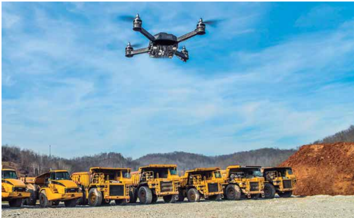
Drone photogrammetry allows superimposing aerial images and converting them into clouds of 3D points.
